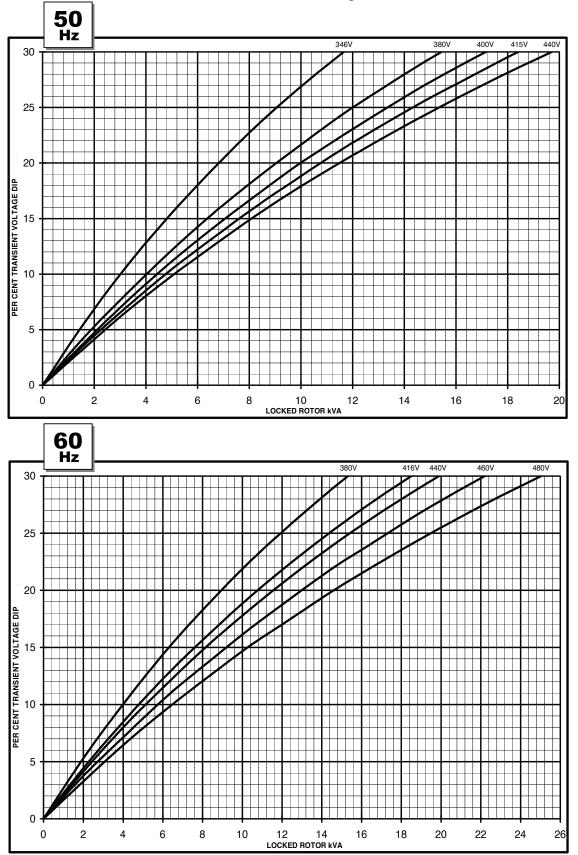
Winding 311 AS480 AVR With EBS fitted Locked Rotor Motor Starting Curves
